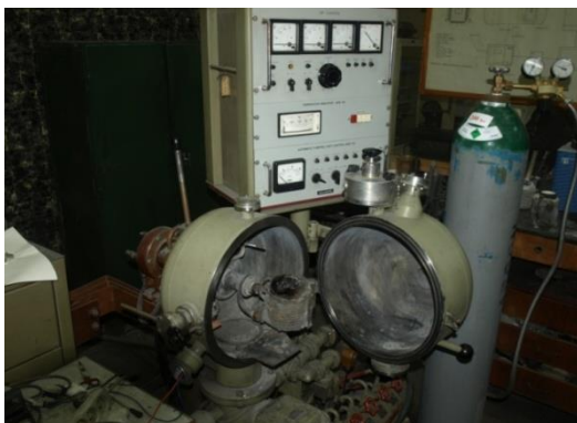
Fig. 2. Laboratory vacuum induction furnace VSG 02 of Balzers company
