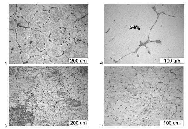
Fig. 6. Microstructure of the Mg-4%Li-1%Ca alloy after casting: a-b) sand mould T=640°C, c-d) sand mould T=690°C, e-f) graphite mould T=690°C, magnification 20x- 200 µm and 50x-100µm
