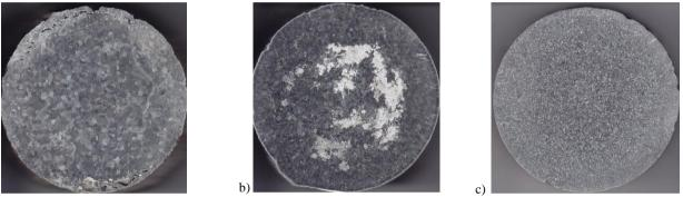
Fig. 4. The macrostructure of the Mg-4%Li-1%Ca alloy after casting: a) sand mould T=640°C, b) sand mould T=690°C, c) graphite mould T=690°C
