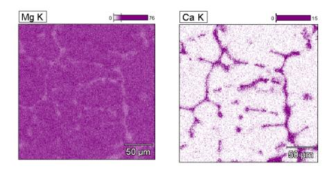
Fig. 8. Surface distribution of Mg and Ca elements in the Mg-4%Li-1%Ca alloy graphite mould T=690°C
