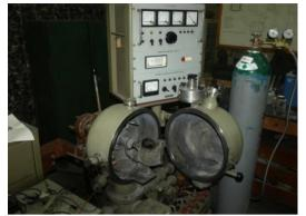
Fig. 2. Laboratory vacuum induction furnace VSG 02 of Balzers company
