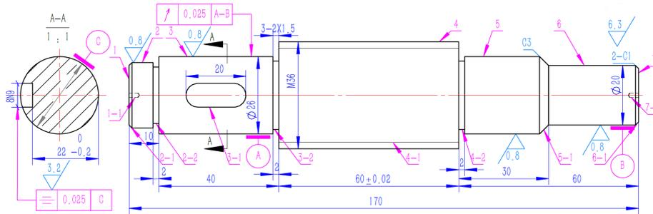
Fig. 4. The model of a transmission shaft
