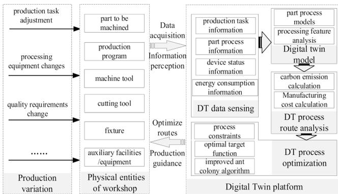
Fig. 2. Dynamic optimization framework of process route based on the digital twin
