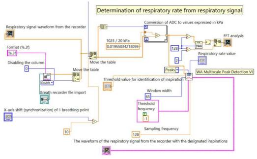
Fig. 4. View of the LabVIEW Block Diagram of the program that extracts inspiration and respiratory rate.
