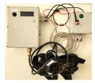
Fig. 3. Proprietary breath recording system using a piezoresistive sensor.
