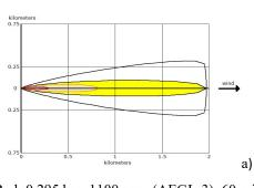
Red: 0,295 km, 1100 ppm (AEGL-3), 60 min Orange: 0,819 km, 160 ppm (AEGL-2), 60 min Yellow: 2.0 km, 30 ppm (AEGL-1), 60 min
