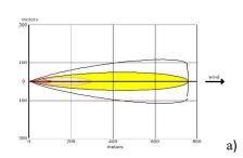
Red: 0,106 km, 1100 ppm (AEGL-3), 60 min Orange: 0,294 km, 160 ppm (AEGL-2), 60 min Yellow: 0,760 km, 30 ppm (AEGL-1), 60 min
