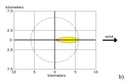
Red: 1.0 km, 1100 ppm (AEGL-3), 60 min Orange: 2.8 km, 160 ppm (AEGL-2), 60 min Yellow: 5.9 km, 30 ppm (AEGL-1), 60 min
