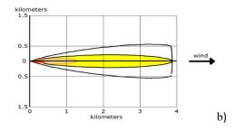
Red:0, 417 km, 1100 ppm (AEGL-3), 60 min Orange: 1.3 km, 160 ppm (AEGL-2), 60 min Yellow: 3.9 km, 30 ppm (AEGL-1), 60 min
