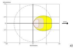
Red: 2.2 km, 1100 ppm (AEGL-3), 60 min Orange: 4.1 km, 160 ppm (AEGL-2), 60 min Yellow: 7.1 km, 30 ppm (AEGL-1), 60 min
