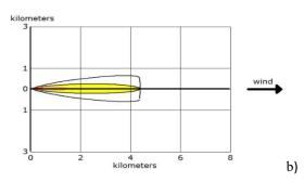
Red: 0,461 km, 1100 ppm (AEGL-3), 60 min Orange: 1.4 km, 160 ppm (AEGL-2), 60 min Yellow: 4.4 km, 30 ppm (AEGL-1), 60 min
