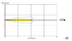
Red: 0,639 km, 1100 ppm (AEGL-3), 60 min Orange: 1.8 km, 160 ppm (AEGL-2), 60 min Yellow: 4.3 km, 30 ppm (AEGL-1), 60 min
