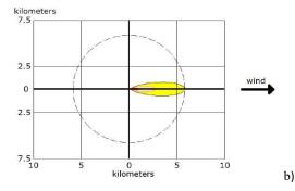
Red: 1.0 km, 1100 ppm (AEGL-3), 60 min Orange: 2.8 km, 160 ppm (AEGL-2), 60 min Yellow: 5.9 km, 30 ppm (AEGL-1), 60 min
