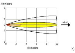
Red: 0,893 km, 1100 ppm (AEGL-3), 60 min Orange: 3.0 km, 160 ppm (AEGL-2), 60 min Yellow: greater than 10 km, 30 ppm (AEGL-1), 60 min
