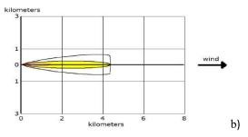
Red: 0,460 km, 1100 ppm (AEGL-3), 60 min Orange: 1.4 km, 160 ppm (AEGL-2), 60 min Yellow: 4.4 km, 30 ppm (AEGL-1), 60 min
