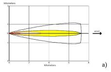
Red: 1.1 km, 1100 ppm (AEGL-3), 60 min Orange: 3.2 km, 160 ppm (AEGL-2), 60 min Yellow: 7.3 km, 30 ppm (AEGL-1), 60 min
