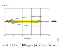
Orange: 3.7 km, 160 ppm (AEGL-2), 60 min Yellow: 8.4 km, 30 ppm (AEGL-1), 60 min
