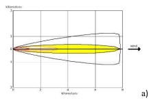
Red: 1.2 km, 1100 ppm (AEGL-3), 60 min Orange: 3.3 km, 160 ppm (AEGL-2), 60 min Yellow: 7.8 km, 30 ppm (AEGL-1), 60 min
