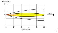
Red: 0,892 km, 1100 ppm (AEGL-3), 60 min Orange: 3.0 km, 160 ppm (AEGL-2), 60 min Yellow: greater than 10 km, 30 ppm (AEGL-1), 60 min
