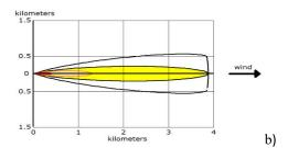
Red: 0,416 km, 1100 ppm (AEGL-3), 60 min Orange: 1.3 km, 160 ppm (AEGL-2), 60 min Yellow: 3.9 km, 30 ppm (AEGL-1), 60 min
