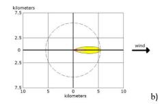
Red: 0,934 km, 1100 ppm (AEGL-3), 60 min Orange: 2.5 km, 160 ppm (AEGL-2), 60 min Yellow: 5.5 km, 30 ppm (AEGL-1), 60 min
