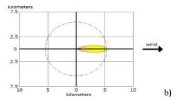
Red: 0,934 km, 1100 ppm (AEGL-3), 60 min Orange: 2.5 km, 160 ppm (AEGL-2), 60 min Yellow: 5.5 km, 30 ppm (AEGL-1), 60 min
