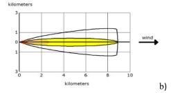
Red: 0,802 km, 1100 ppm (AEGL-3), 60 min Orange: 2.7 km, 160 ppm (AEGL-2), 60 min Yellow: 8.9 km, 30 ppm (AEGL-1), 60 min
