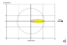
Red: 0,539 km, 1100 ppm (AEGL-3), 60 min Orange: 1.2 km, 160 ppm (AEGL-2), 60 min Yellow: 2.3 km, 30 ppm (AEGL-1), 60 min
