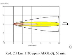
Orange: 5.4 km, 160 ppm (AEGL-2), 60 min Yellow: greater than 10 km, 30 ppm (AEGL-1), 60 min
