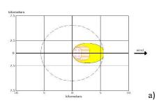
Red: 1.6 km, 1100 ppm (AEGL-3), 60 min Orange: 3.1 km, 160 ppm (AEGL-2), 60 min Yellow: 5.6 km, 30 ppm (AEGL-1), 60 min
