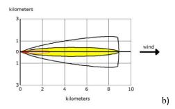
Red: 0,802 km, 1100 ppm (AEGL-3), 60 min Orange: 2.7 km, 160 ppm (AEGL-2), 60 min Yellow: 8.9 km, 30 ppm (AEGL-1), 60 min
