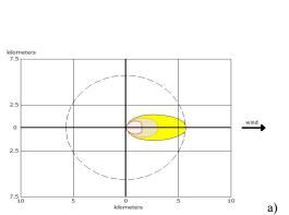
Red: 1.5 km, 1100 ppm (AEGL-3), 60 min Orange: 3.0 km, 160 ppm (AEGL-2), 60 min Yellow: 5.7 km, 30 ppm (AEGL-1), 60 min
