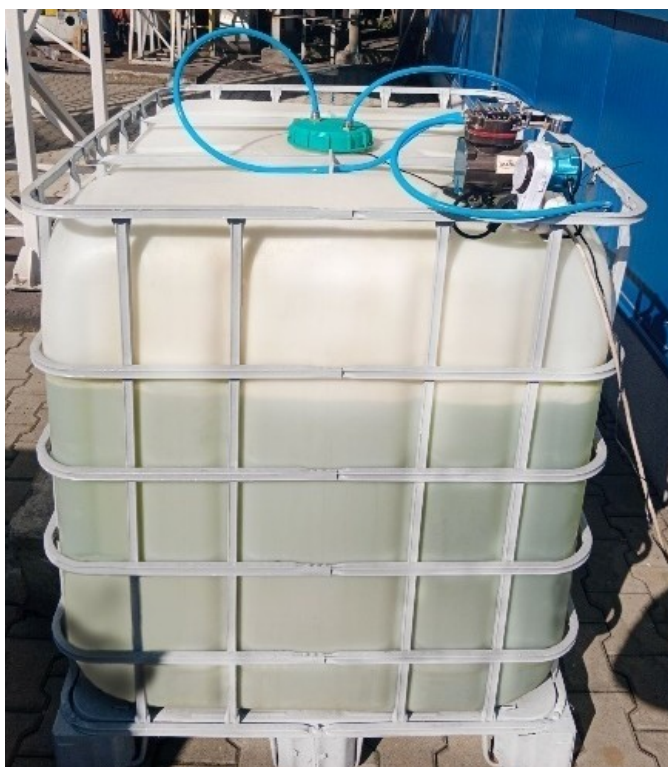
Figure 3. Installation for absorbing carbon dioxide using Chlorella vulgaris algae in industrial conditions.
