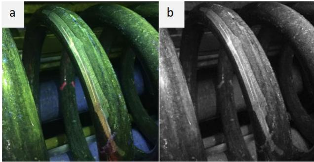
Fig. 6. a) Original image with crack on surface, b) grayscale image
