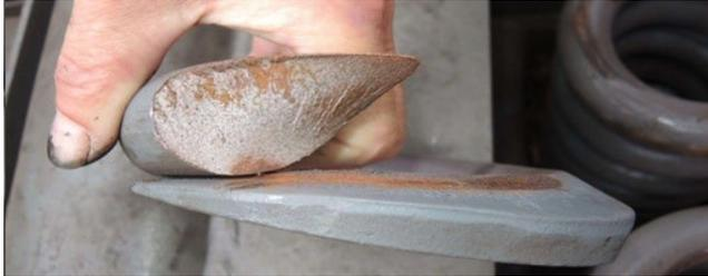
Fig. 1. Locomotive bogie spring fracture example [9]
