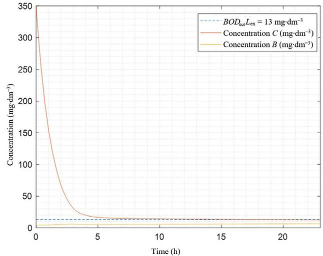
**Fig. 2.** Distribution of pollution and activated sludge concentration during the day for scenario 1;  $C$  = concentration of pollution in the filter ( $\text{mg} \cdot \text{dm}^{-3}$ ),  $B$  = concentration of activated sludge in the reactor ( $\text{mg} \cdot \text{dm}^{-3}$ ),  $BOD_{\text{out}}L_{\text{ex}}$  = biochemical oxygen demand at the aeration tank outlet; source: own study
