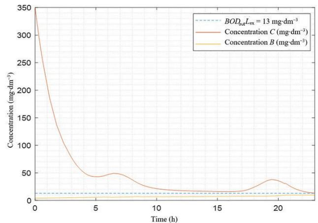
**Fig. 4.** Distribution of pollution and activated sludge concentration during the day for scenario 3;  $C$ ,  $B$ ,  $BOD_{\text{out}}L_{\text{ex}}$  as in Fig. 2; source: own study
