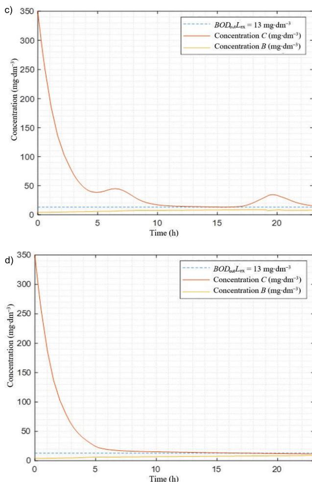
Fig. 6. Distribution of pollution and activated sludge concentration during the day for scenario 3 with an increase in air supply to the aeration zone: a)  $K = 0.5 \text{ mg}\cdot\text{dm}^{-3}$ , b)  $K = 1 \text{ mg}\cdot\text{dm}^{-3}$ , c)  $K = 1.5 \text{ mg}\cdot\text{dm}^{-3}$ , d)  $K = 2 \text{ mg}\cdot\text{dm}^{-3}$ ;  $K$  as in Fig. 5,  $C$ ,  $B$ ,  $BOD_{\text{out}}$   $L_{\text{ex}}$  as in Fig. 2; source: own study
