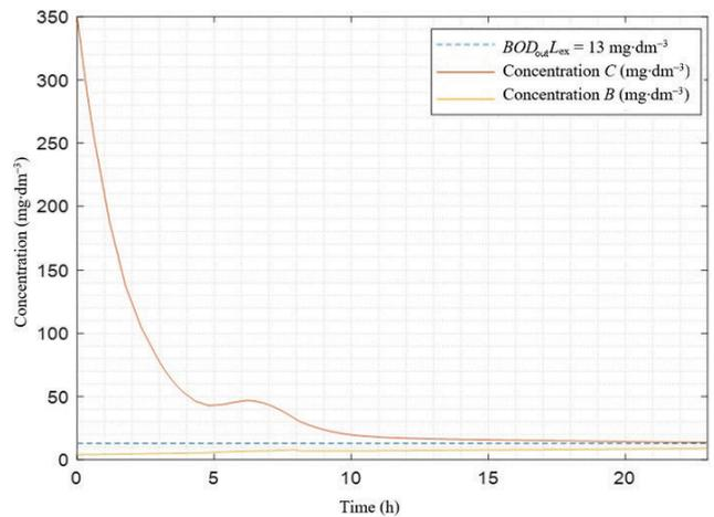
**Fig. 3.** Distribution of pollution and activated sludge concentration during the day for scenario 2;  $C$ ,  $B$ ,  $BOD_{\text{out}}L_{\text{ex}}$  as in Fig. 2; source: own study
