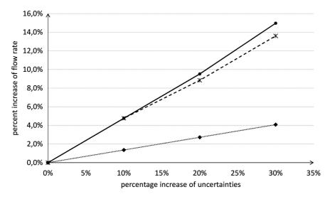
Fig. 4. The dependence of the influence of the percentage change of the uncertainty of roughness coefficients of the channel, of the floodplain, and of the uncertainty of the geometric dimensions of the river channel water area on the uncertainty of the discharge
