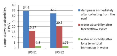
Fig. 8. Comparison of dampness level in EPS boards collected from an inverted roof, resulting from various operational loads
