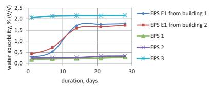
Fig. 6. Increase in the EPS boards' water absorbability during total immersion in water at  $(23 \pm 2)^{\circ}$ C for 28 days
