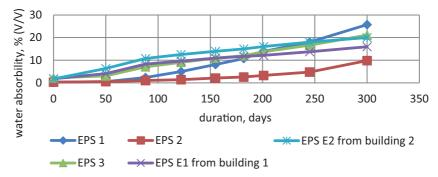
Fig. 7. Increase in EPS boards' water absorbability after 300 freeze/thaw cycles and previous total immersion of the boards in water at  $(23 \pm 2)^{\circ}$ C for 28 days
