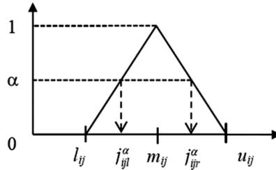
Fig. 4.  $\alpha$ -cut index and triangle fuzzy number [16]
