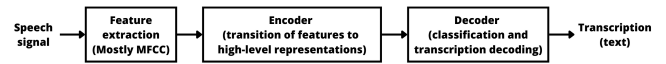
Fig. 2. A simplified diagram of the ASR system in the E2E approach, in which acoustic, language and pronunciation models are implemented by an integrated deep model that requires soft audio and transcript alignment [9].
