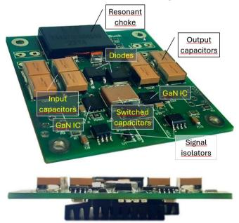
$\mbox{Fig.3.}$  The laboratory converter implementation: top view on components and side view with heatsinks
