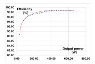
Fig.5. Results of the efficiency of the converter
