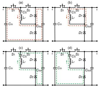
**Fig.2.** Stages of operation: (a) and (c): operation with one transistor turned-on, (b) and (d): current passing during the dead-time and reverse conduction of a transistor
