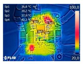
**Fig.7.** Results of the thermal imaging measurements of the converter at  $P_{out} = 400 \text{ W}$ ,  $f_s = 400 \text{ kHz}$  and forced air flow with an ambient temperature of 20 degrees Celsius (measurement points Sp1, Sp2 indicates transistors and Sp3, Sp4 diodes).
