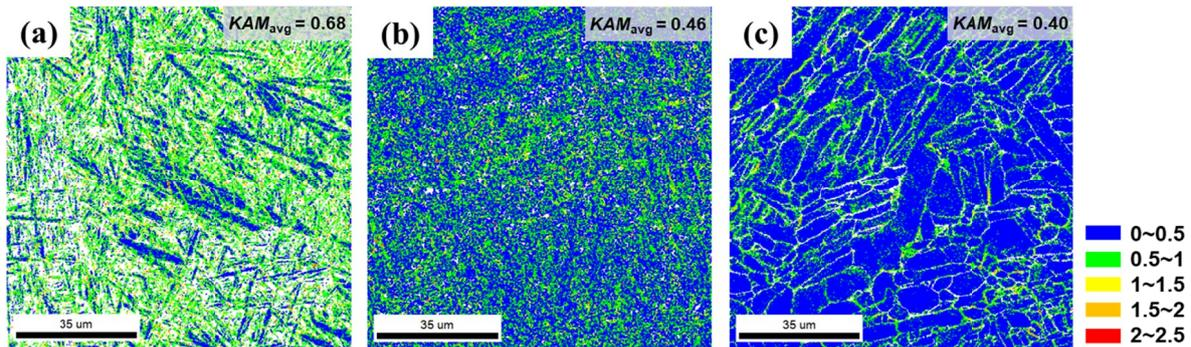
Fig. 3. EBSD KAM maps of SLMed Ti-6Al-4V alloy after different heat treatments including (a) SLMed, (b) annealing and (c) HIP
