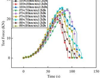
(c) Different process parameters (P = 975 W, V = 800 mm/min) Fig. 6. Force evolution curves for different deformation amplitudes (a), fillet radii (b), and process parameters (c)
