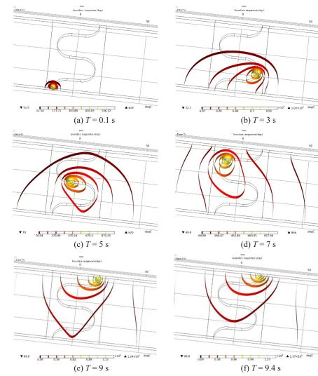
Fig. 3. Temperature field at different times
