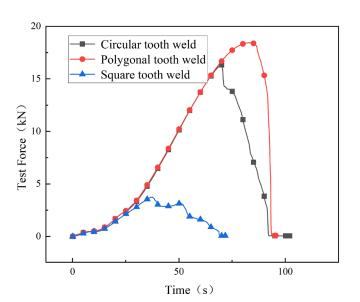
Fig. 5. Force-time curve of the curve path tensile test (a = 20 mm, T = 40 mm, r = 3 mm)
