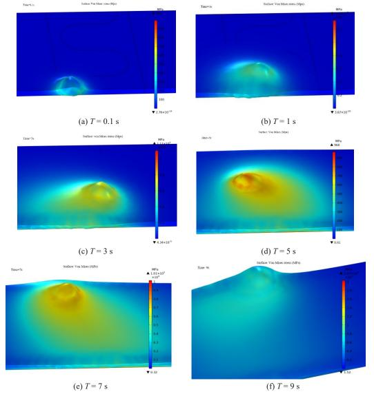
Fig. 4. Thermal stress distribution at different time locations under the same group of paths
