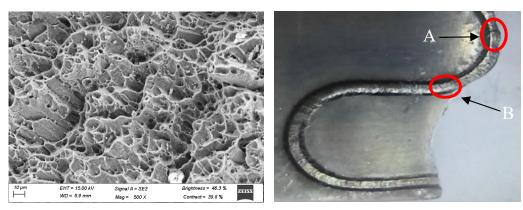
(a) Tensile fracture of the 6063-T6 base material
