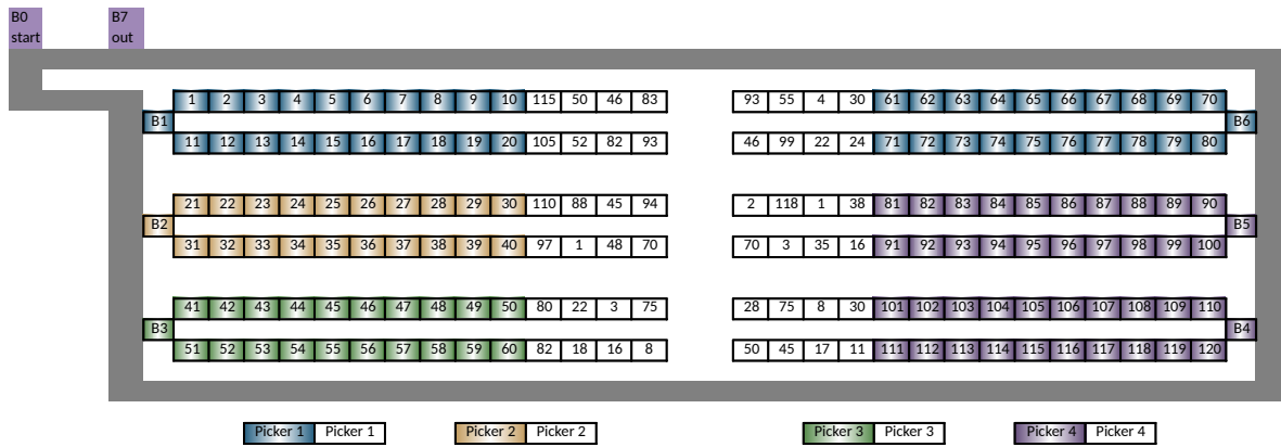
Fig. 2. The layout of a distribution center in which a picker completes orders in several buffers: B0 – start buffer; B7 – out buffer; B1-B6 – order picking buffers; Dark colors in buffers B1-B6 – regular buffer products; Light colors in buffers B1-B6 – products also allocated in other buffers
