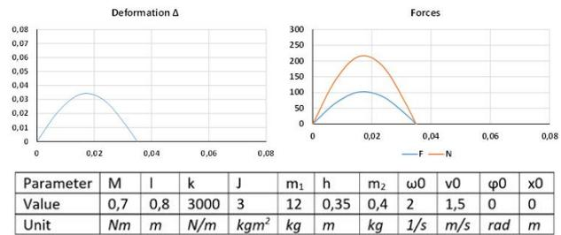
Fig. 11. Simulation results – experiment 2
