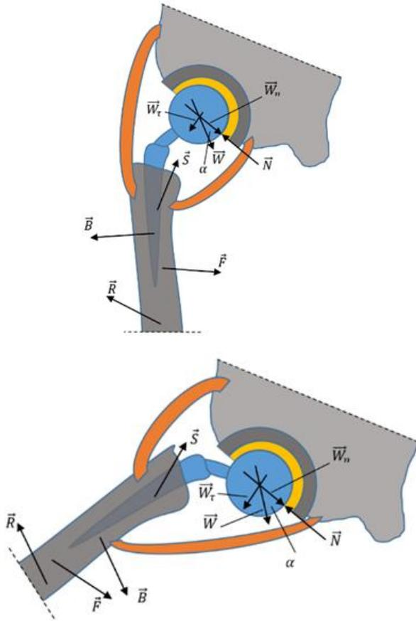
Fig. 6. Forces in an unstable system – various limb positions
