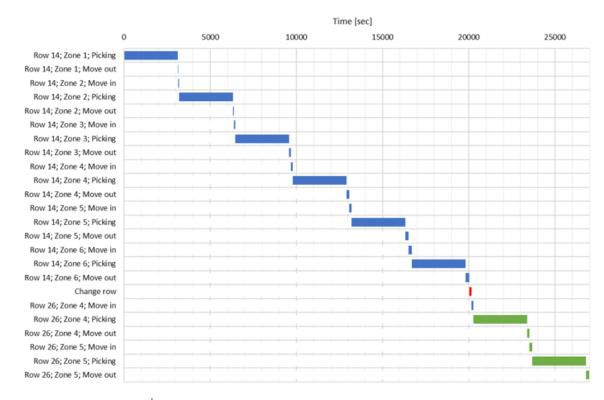
Fig. 15. Gant-diagram for  $3^{rd}$  type pickers picking a full row and Zone4-Zone 5 in a second row (for pickers ID13-18)
