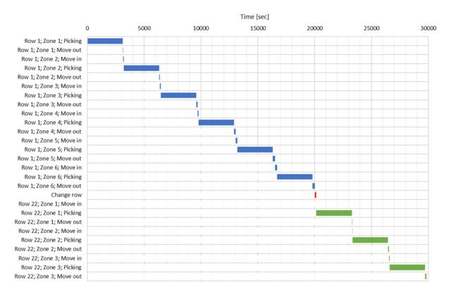
Fig. 13. Gant-diagram for  $1^{st}$  type pickers picking a full row and Zone1-Zone 3 in a second row (for pickers ID01-09)
