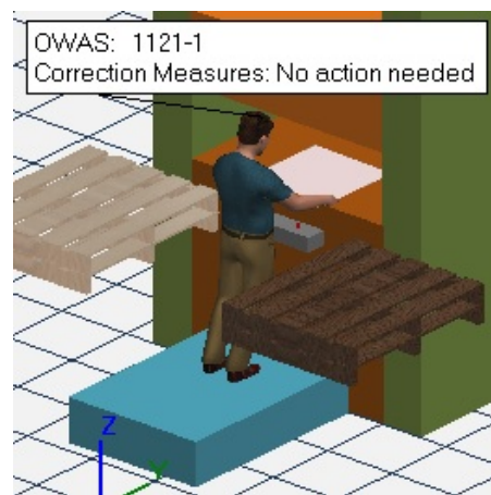
Fig. 10. Placing the metal sheet in the press after ergonomic intervention
