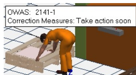
Fig. 5. Placing the stamped metal sheet on the pallet
