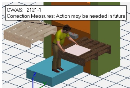
Fig. 9. Picking up a metal sheet after ergonomic intervention
