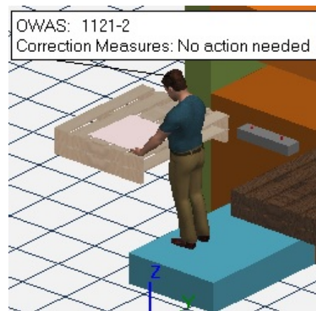
Fig. 11. Placing a metal sheet on a pallet after ergonomic intervention
