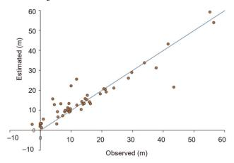
Fig. 4. Computed versus observed depth to groundwater using IDW interpolation for a random 50 datapoints; source: own study
