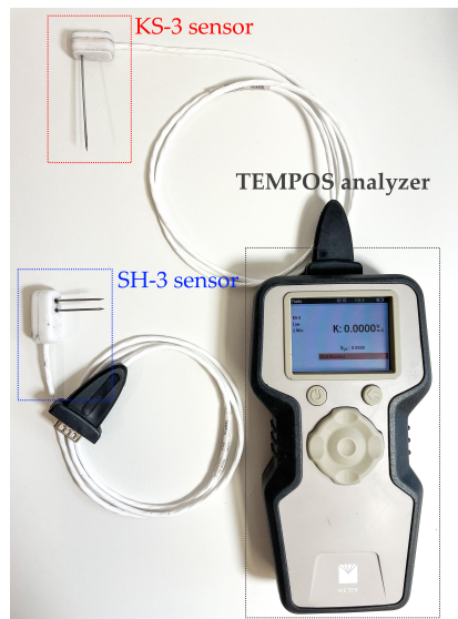
Figure 1: A commercial device used in the research to measure the thermal conductivity of base PCM and NEPCM using the transient hot wire method.
