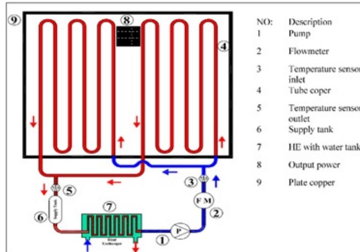
Figure 8: Schematic diagram of two passes fluid circulation in PV/T system [73].
