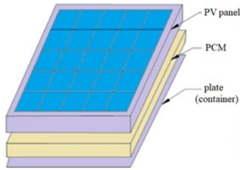
Figure 11: PCM installation in PV panel [104].
