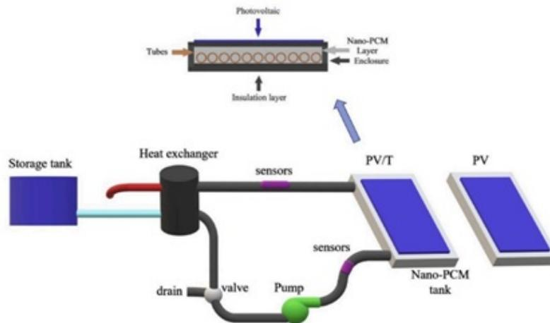
Figure 13: A schematic diagram of the PV/T system and a cross-section of the collector [36].
