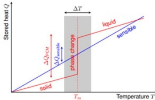
Figure 12: Thermal behaviour of PCM [106].
