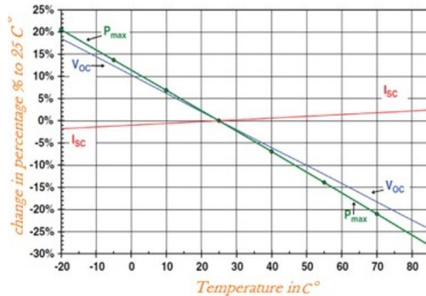
Figure 4: The change of  $V_{oc}$ ,  $P_{\max}$ , and  $I_{sc}$  with temperature [13].
