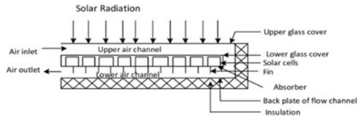
Figure 9: Cross-sectional view of double-pass air photovoltaic panel with fins [77].
