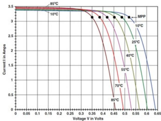
Figure 3: The change in voltage and current with temperatures as a parameter [13].
