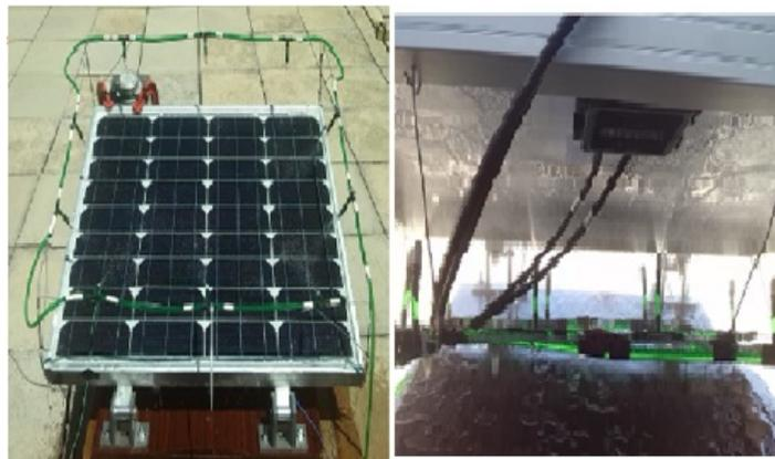
Figure 6: Cooling the front and the backside of the photovoltaic panel [67].
