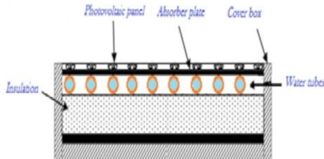
Figure 5: Cross section of photovoltaic panel water cooling [59].
