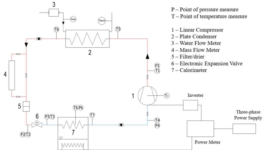
Figure 1: Scheme 2D of the experimental stand.
