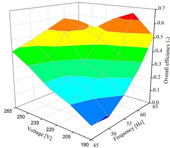
Figure 7: The overall efficiency of a linear compressor against the supply frequency and voltage.
