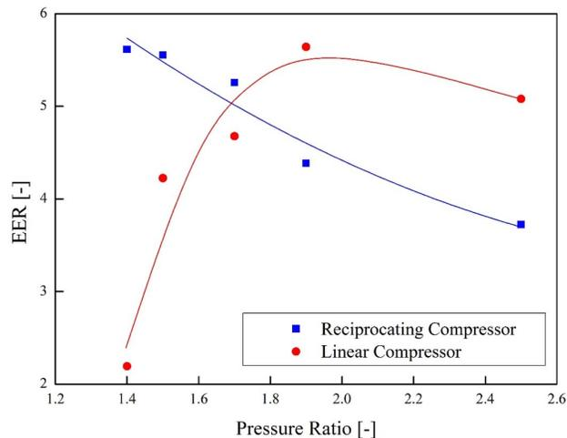
Figure 12: EER of the refrigeration system against the pressure ratio.
