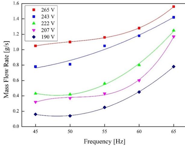
Figure 5: The mass flow rate of a linear compressor against the frequency of the supply current.
