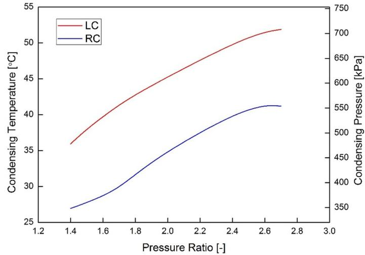
Figure 3: Compressors condensing temperatures and pressures during the second stage of research.
