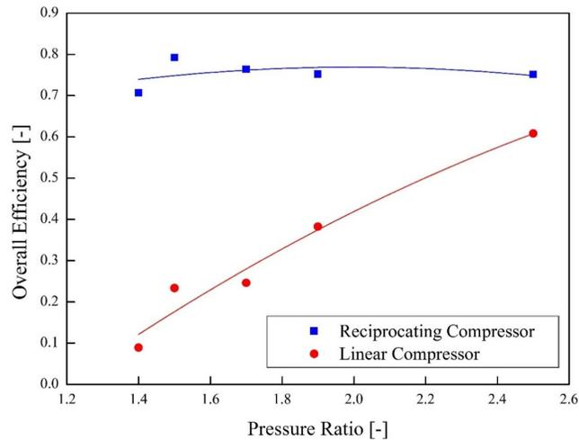
Figure 11: Compressor efficiency against the pressure ratio.
