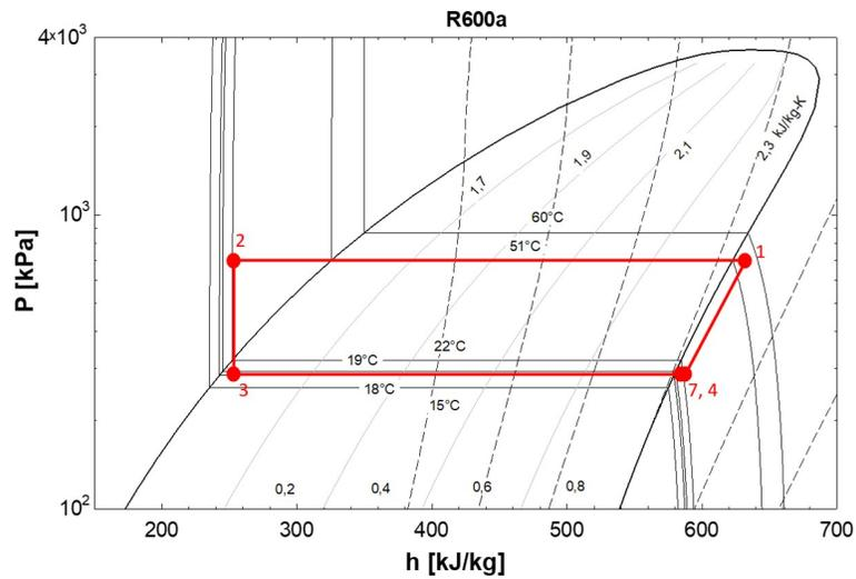
Figure 4: Refrigeration cycle of the tested system in the  $p-h$  coordinate system.
