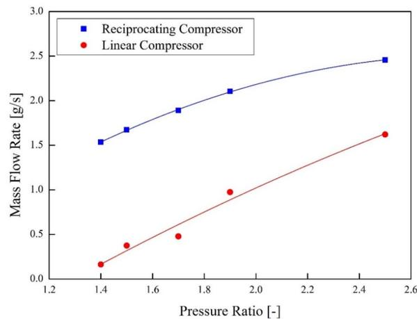
Figure 9: The mass flow rate of a linear compressor and reciprocating compressor against the pressure ratio.
