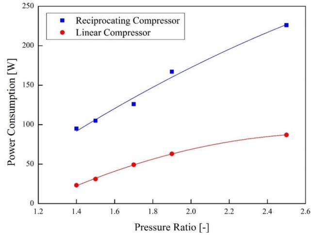
Figure 10: Electric power consumption of the compressor against the pressure ratio.
