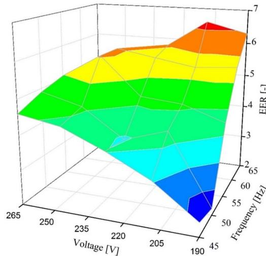
Figure 8: EER of the refrigeration system against the supply frequency and voltage of the linear compressor.
