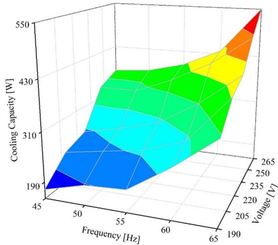
Figure 6: The cooling capacity of a linear compressor against the frequency and voltage of the supply current.
