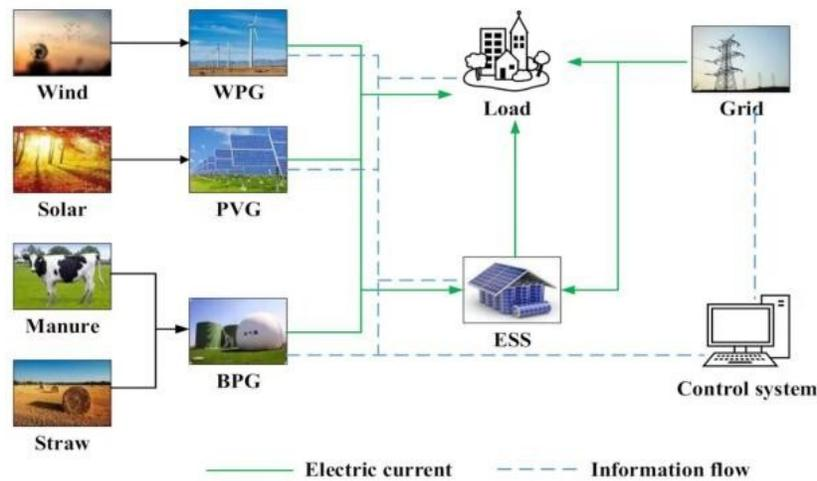
Figure 3: Wind-solar-biomass hybrid energy system: WPG – wind power generator, PVG – photovoltaic generators, BPG – biomass generator, ESS – energy storage system.
