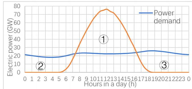
Figure 1: Averaged daily grid demand curve and solar power generation curve in Australia.
