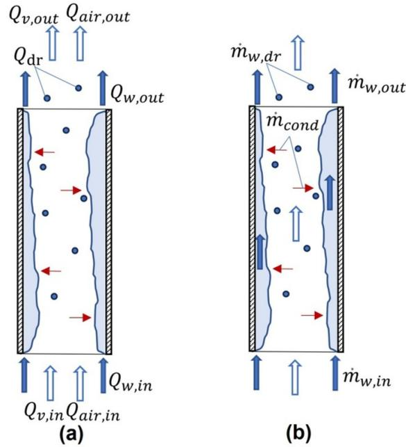
Figure 2: (a) Energy balance. (b) Water mass balance.
