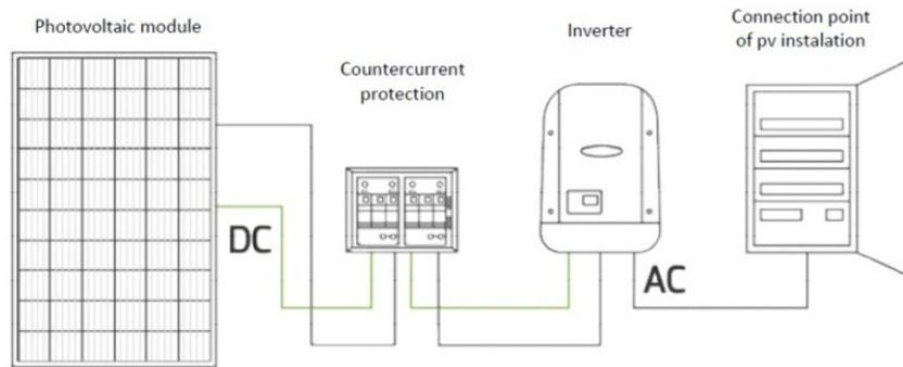
Figure 1: Schematic diagram of the photovoltaic system: DC – direct current, AC – alternating current [6].
