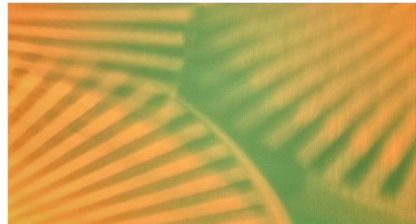
**Fig. 11.** Three identical, shifted images reflecting Siemens-star test pattern (72 sectors, #58-833 Edmund Optics Ltd.)
