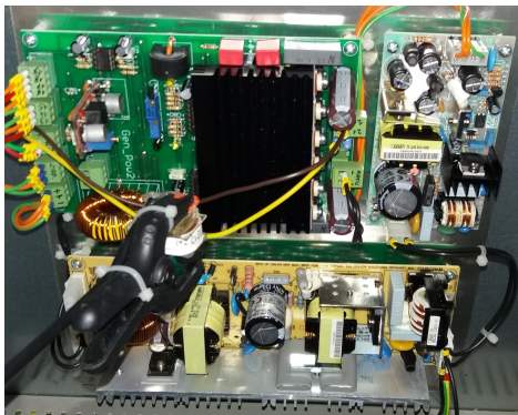
Fig. 14. The view of the inverter of the 160 W 40 kV used for electrostatic segregation [8]
