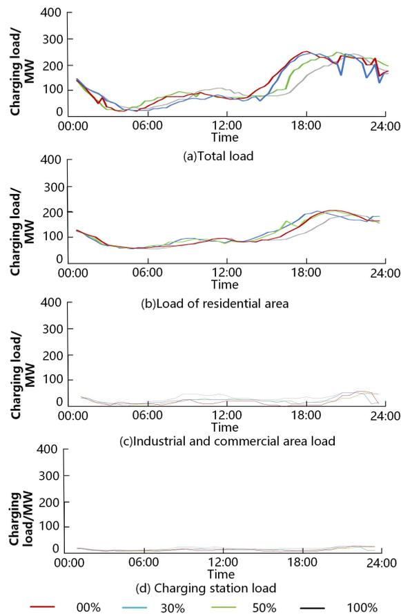
Fig. 4. Charging load of different charging facilities
