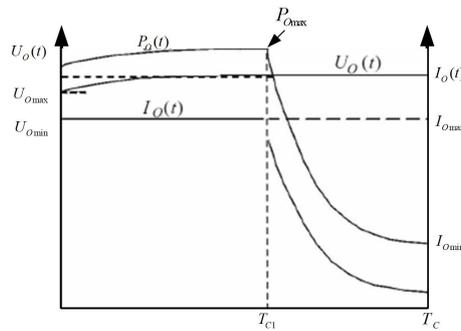
Fig. 1. Variation of charging power of EV with time
