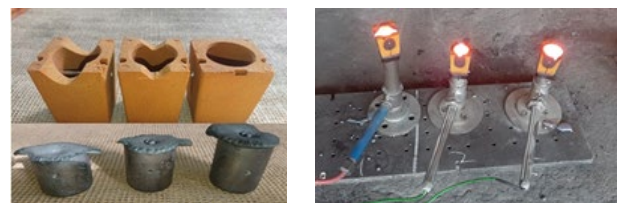
Fig. 10. a/ AT samplers filled to the height, h: 28.0, 34.0 and 40.0mm and with the geometric solidification modulus, M: 0.52, 0.56 and 0.60cm, b/ the stand of pouring AT samplers
