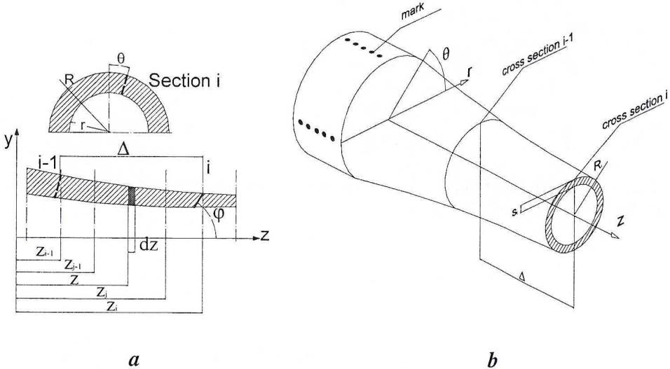
Fig. 1. a) Pins deformations in cross-sections  $i$  (actual) and  $i-1$  (conventional) including stroke volume (in general, the  $i-1$  and  $i$  cross-sections are located between the  $j-1$  and  $j+1$  control cross-sections), b) The working cone with the pins marked
