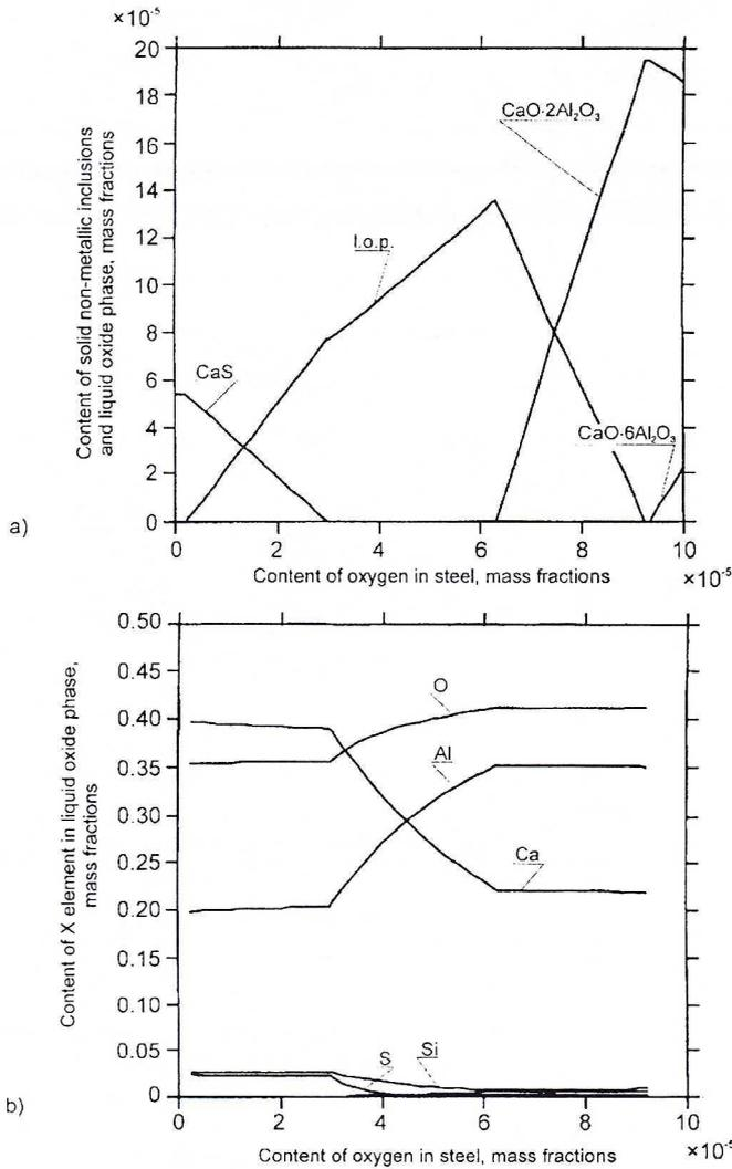
Fig. 3. Influence of total oxygen content in steel with the following chemical composition: 0.2% C, 0.8% Mn, 0.25% Si, 0.02% Al, 0.01% S, 0.003% Ca on non-metallic inclusion precipitation process in steel bath at 1873 K: a) type and content of non-metallic inclusions (l.o.p. – liquid oxide phase), b) chemical composition of liquid oxide phase
