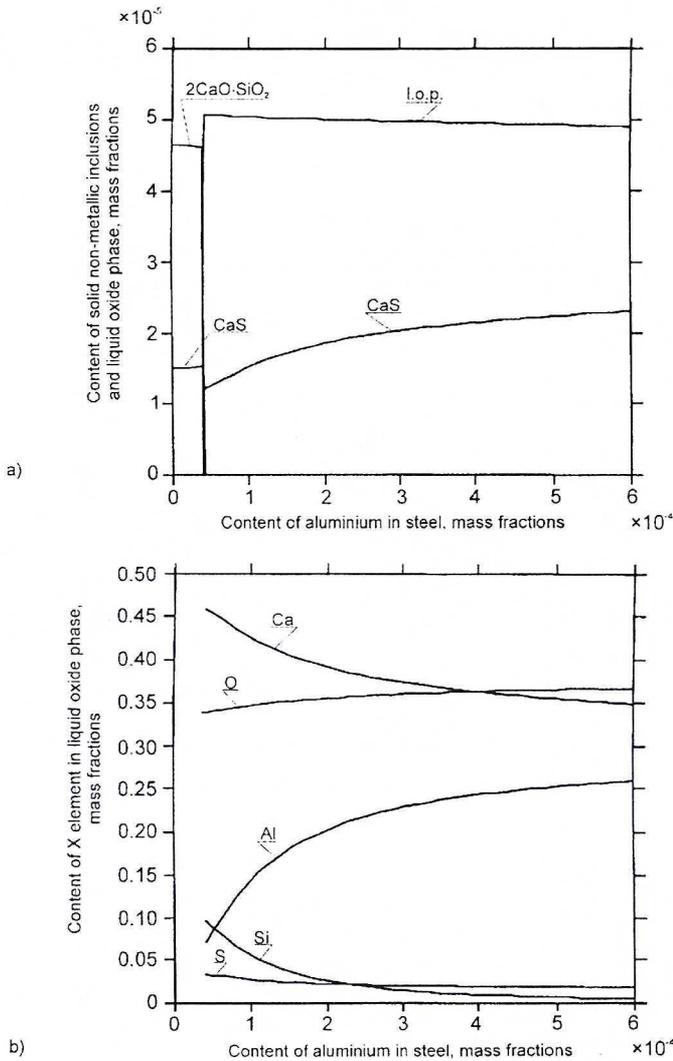
Fig. 4. Influence of aluminium content in steel with the following chemical composition: 0.2% C, 0.8% Mn, 0.25% Si, 0.01% S, 0.002% O<sub>T</sub>, 0.003% Ca on non-metallic inclusion precipitation process in steel bath at 1873 K:
