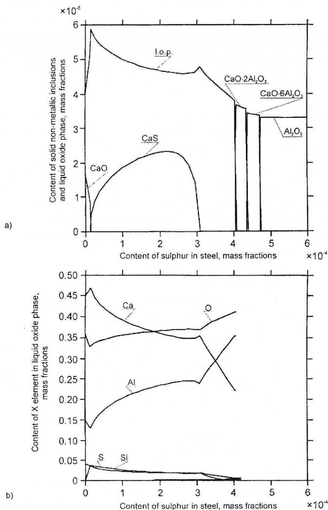
Fig. 2. Influence of sulphur content in steel with the following chemical composition: 0.2% C, 0.8% Mn, 0.25% Si, 0.02% Al, 0.002% O<sub>T</sub>, 0.003% Ca on non-metallic inclusion precipitation process in steel bath at 1873K: a) type and content of non-metallic inclusions (I.o.p. – liquid oxide phase), b) chemical composition of liquid oxide phase
