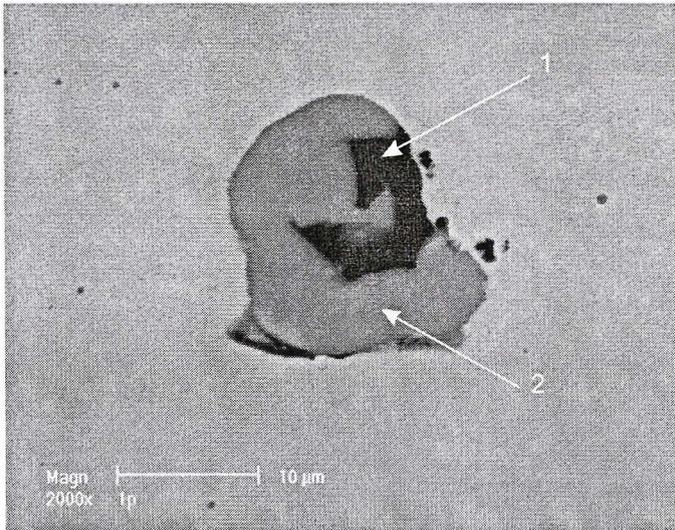
Fig. 11. Oxide-sulphide inclusion in 22HNMhD steel, heat 78504, sample "1p" from hot rolled bar; 1 –  $\text{CaO} \cdot 6\text{Al}_2\text{O}_3$ -type calcium aluminate, 2 –  $(\text{Mn,Ca})\text{S}$  sulphide with small Ca content
