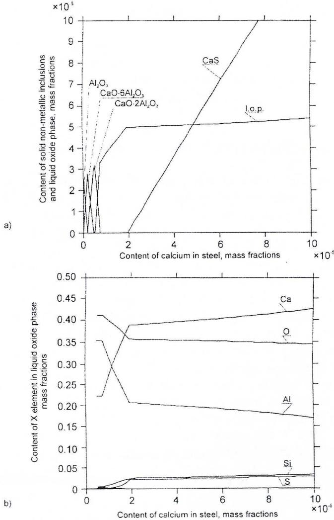
Fig. 1. Influence of calcium content in steel with the following chemical composition: 0.2% C, 0.8% Mn, 0.25% Si, 0.02% Al, 0.01% S, 0.002%  $O_T$ , on non-metallic inclusion precipitation process in steel bath at 1873K: a) type and content of non-metallic inclusions (I.o.p. – liquid oxide phase), b) chemical composition of liquid oxide phase
