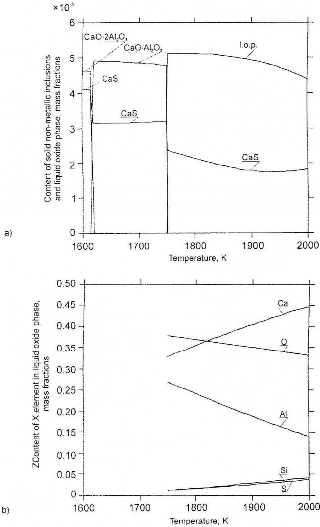
Fig. 5. Influence of temperature of steel bath with the following chemical composition: 0.2% C, 0.8% Mn, 0.25% Si, 0.02% Al, 0.01% S, 0.002% O<sub>T</sub>, 0.003% Ca on non-metallic inclusion precipitation process:
