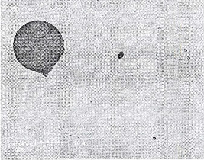
Fig. 7. Calcium aluminate of  $2\text{CaO} \cdot \text{Al}_2\text{O}_3$ -type in 080M40 steel, heat 29495, sample A4 taken after the first portion of calcium is added
