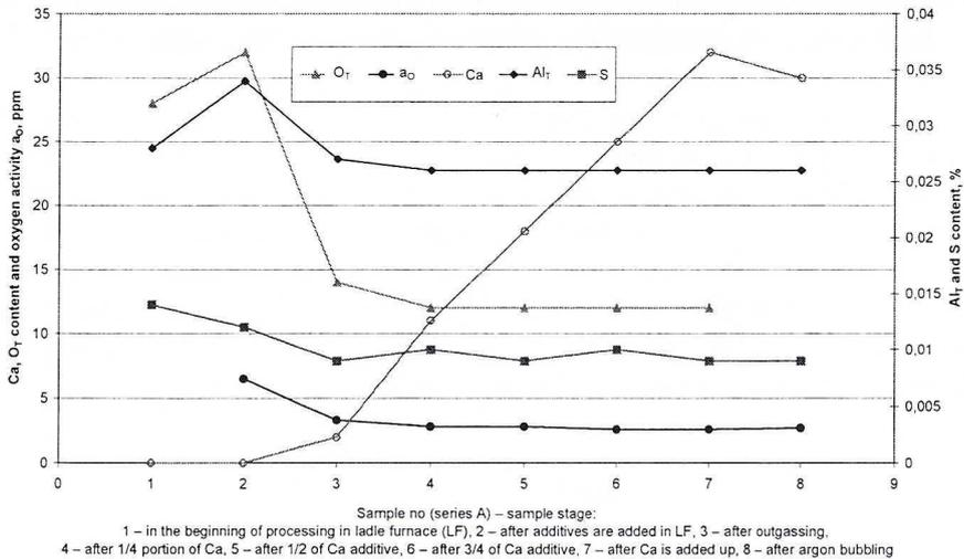
Fig. 6. Changes in chemical composition of steel bath during ladle processing of 080M40 steel, heat 29495
