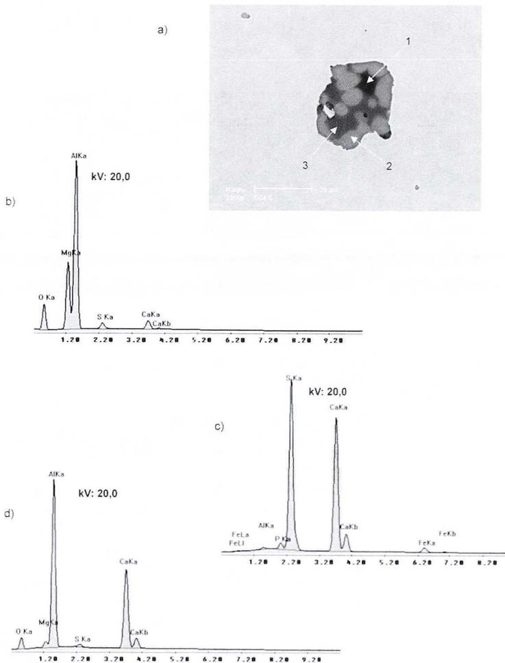
Fig. 10. Complex oxide-sulphide inclusion in 22HNMhD steel, heat 78504, sample 5; microscopic image (a) and chemical composition analysis in point: 1 –  $2\text{Al}_2\text{O}_3 \cdot \text{MgO}$  (b), 2 –  $\text{CaS}$  (c), 3 –  $\text{Al}_2\text{O}_3 \cdot \text{CaO}$  + trace of  $\text{MgO}$  (d)
