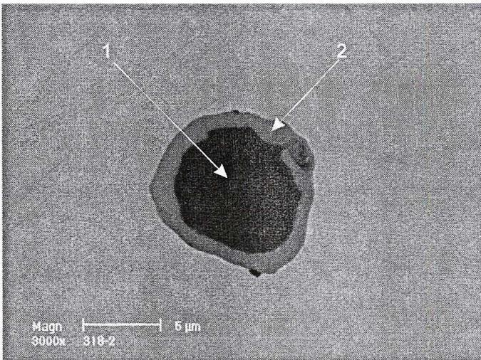
Fig. 8. Oxide-sulphide inclusion in 871M40 steel
