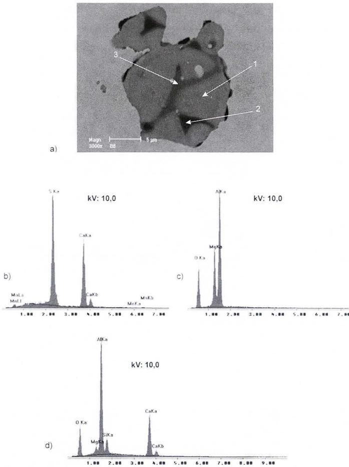
Fig. 9. Oxide-sulphide inclusion in 080M40 steel heat 29590, sample B8 taken after calcium is added: microscopic image (a) and results of chemical composition analysis in point:
