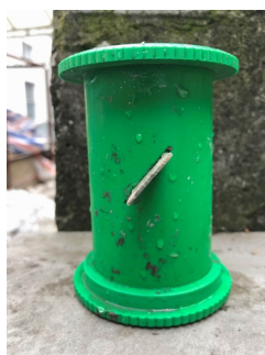
Fig. 1. Mold for making sandstone like samples with cracks
