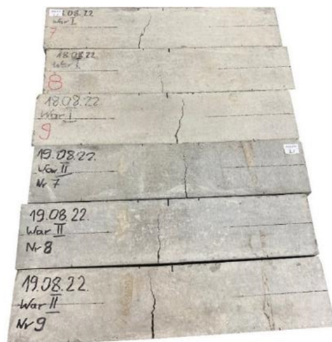
Fig. 12. Samples 7-9 from concrete of Type 1 and 2 after the 4PBT – quasi-vertical crack between the upper supports
