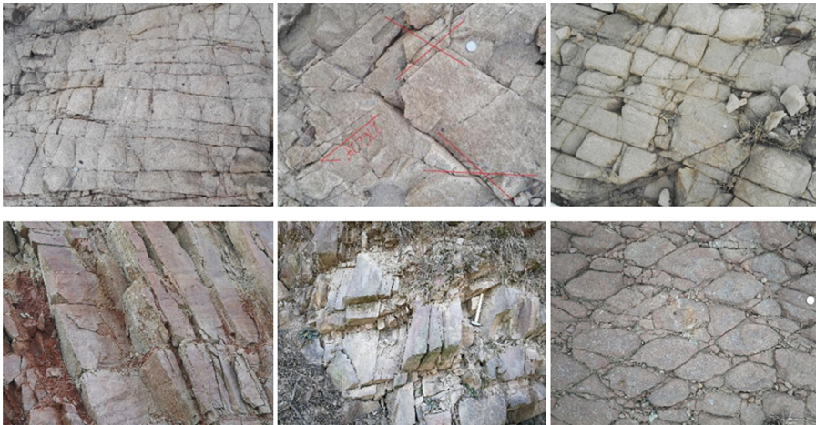
Fig. 4. Conjugate shear joint diagram of field test points
