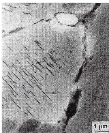
Fig. 8. TEM micrograph of the Al-Cu 4-Mg 1.8-Mn 0.7-Fe 1-Ni 1.5-Zr 0.25 alloy after recrystallization showing precipitates of intermetallic compounds lying in the grain boundaries
