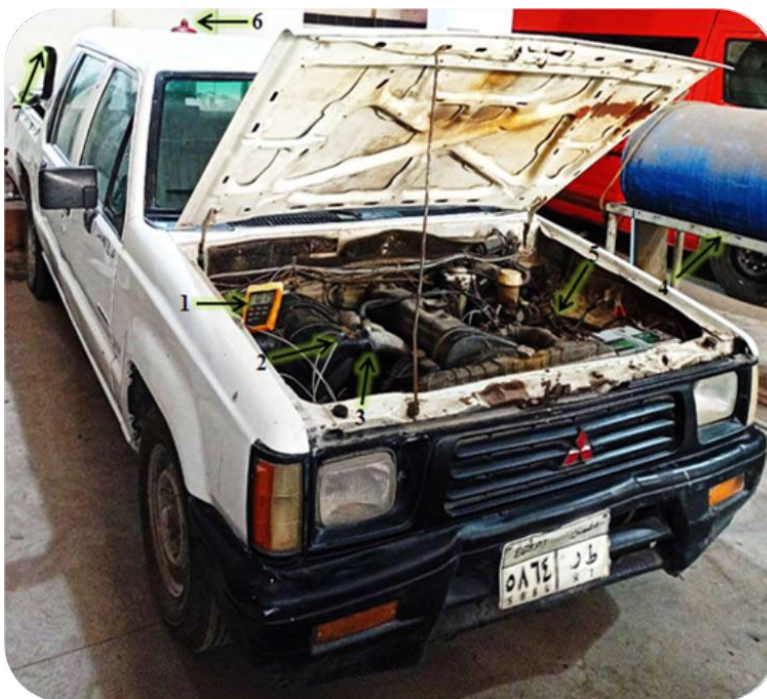
(b) Front view of the modified vehicle showing measuring devices
