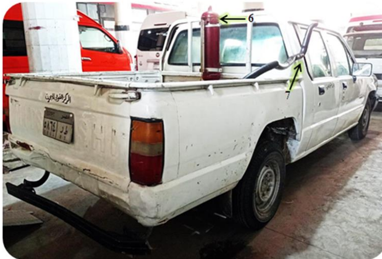
(a) Back view of the tested vehicle showing exhaust and fuel systems
