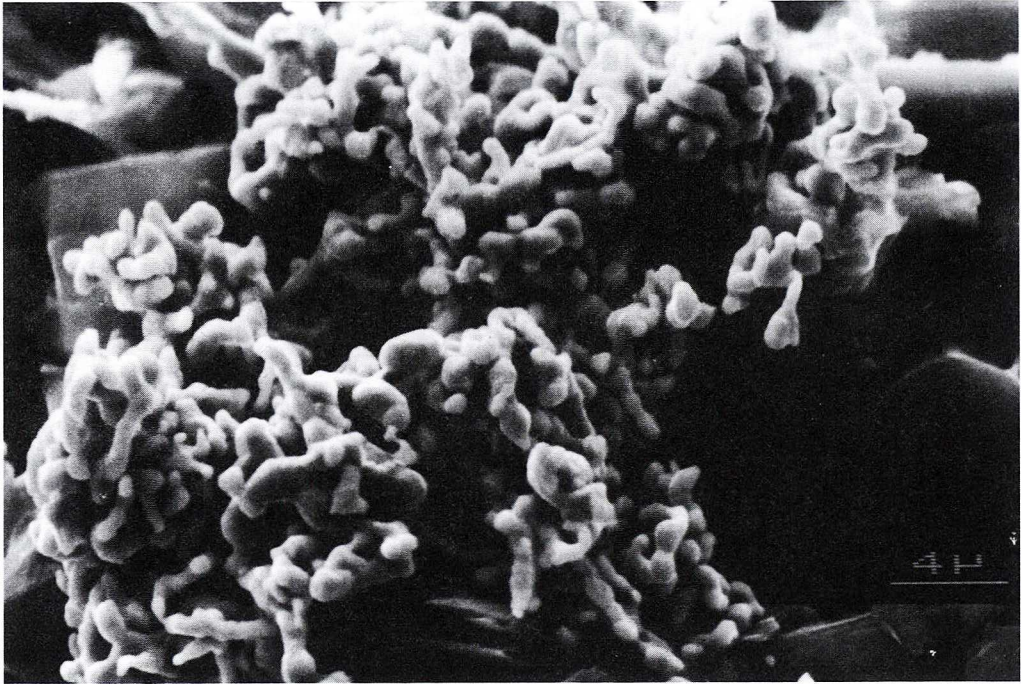
Fig. 2. SEM micrograph of extrafine cobalt powder with fibre shaped structure
