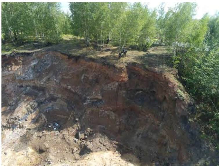
Fig. 2. Exposed slope of zinc waste dump in Ruda Śląska – Bykowina (photo A. Bartela)
