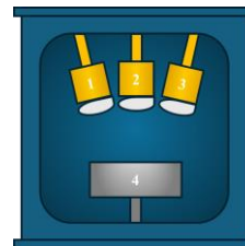
Fig.1. Location of samples in relation to the magnetron guns in the chamber (1, 3 - magnetron guns; 2 - plasma gun; 4 - sample table)
