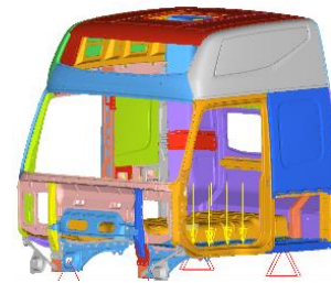
Fig. 3. Bending working condition model
