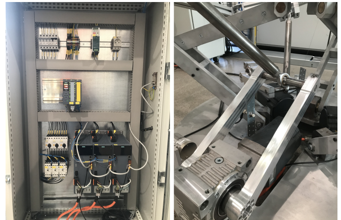
Fig. 6. Control and executive elements of the platform [36]
