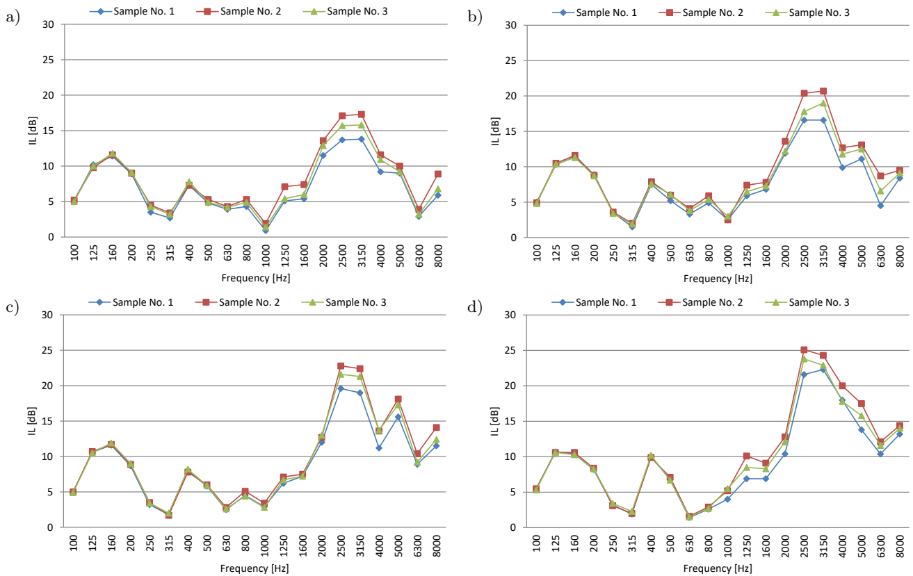
Fig. 10. Results of louvers' insertion loss with different tilt angles of plates away from the source: a) 0°; b) 15°; c) 30°; d) 45°.
