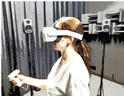
Fig. 4. Tested person wearing VR goggles during an auditory test at the Auralization Laboratory at AGH University of Science and Technology.
