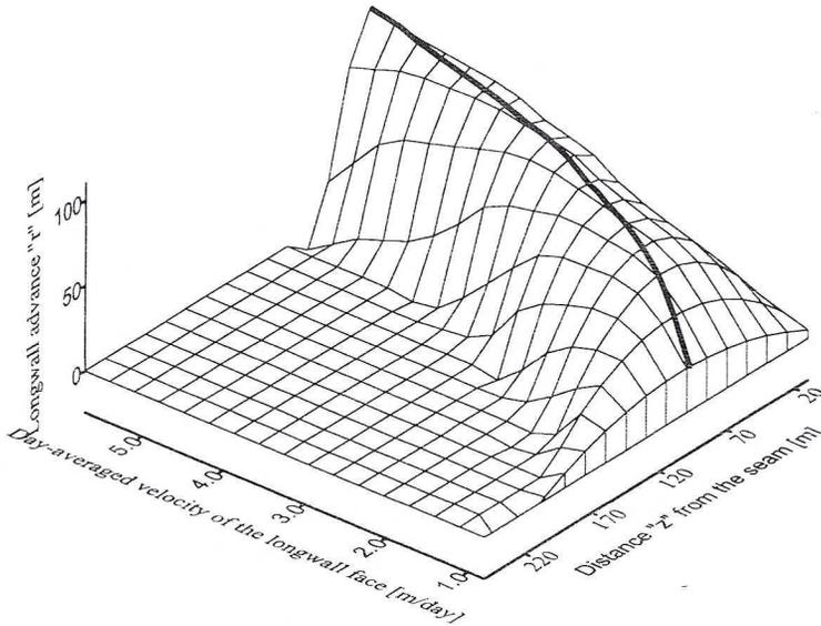
Fig. 5. Graphic illustration of the active volume of the rock mass for given average longwall face advance rates in the range from 0.5 m/day to 6.0 m/day
