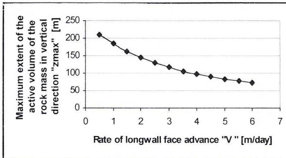
Fig. 2. Graph of function  $z_{\max} = f(V)$  for the face advance rate range from 0.5 m/day to 6.0 m/day
