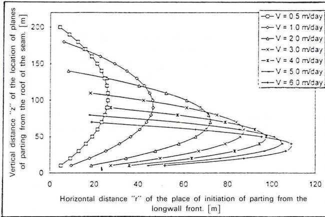
Fig. 1. Curves presenting the locations of initiation of the rock mass parting planes for given longwall face advance rates (Drzewiecki, 1977)
