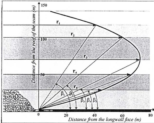
Fig. 4. Cross-section throughout the longwall environment with indication of position of the rock mass parting planes for an average rate of face advance of 2 m/day
