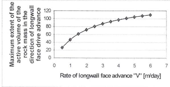
Fig. 3. Graph of function  $r = f(V)$  for the face advance rate range from 0.5 m/day to 6.0 m/day
