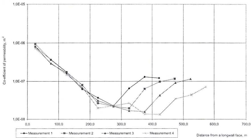
Fig. 7. Change in co-efficient of permeability of caving zone depending on the distance from a longwall face 765
