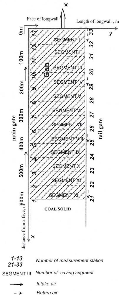
Fig. 1. U-advancing ventilation system of a longwall
