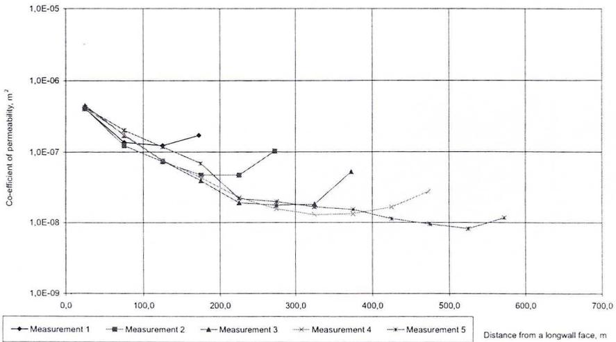
Fig. 5. Change in co-efficient of permeability of caving zone depending on the distance from a longwall face 660
