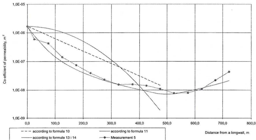
Fig 12. Change in co-efficient of permeability of caving zone for the last series together with approximation for longwall 220
