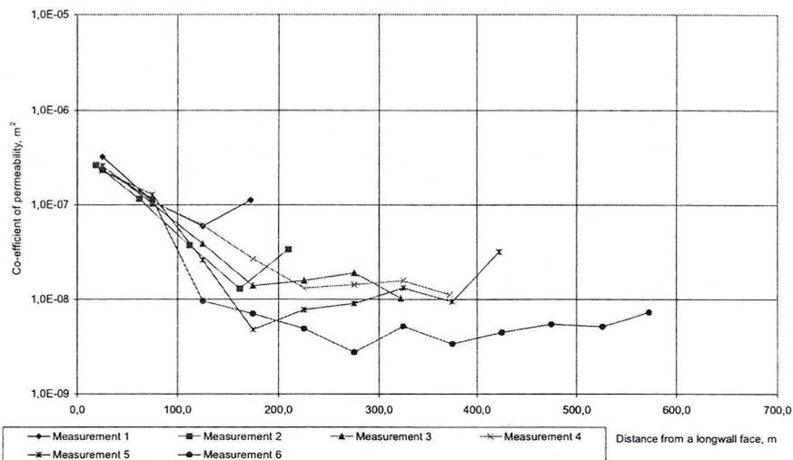
Fig. 2. Change in co-efficient of permeability of caving zone depending on the distance from a longwall face 465
