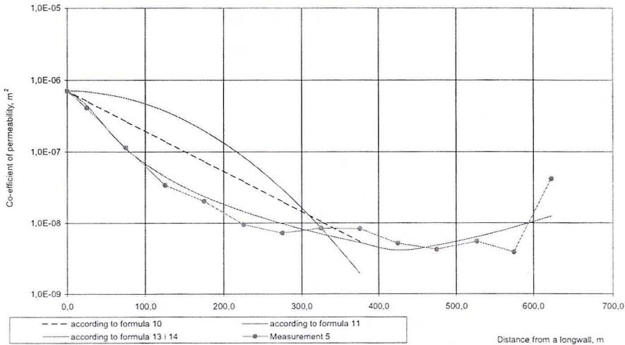
Fig. 9. Change in co-efficient of permeability of caving zone for the last series together with approximation for longwall 405
