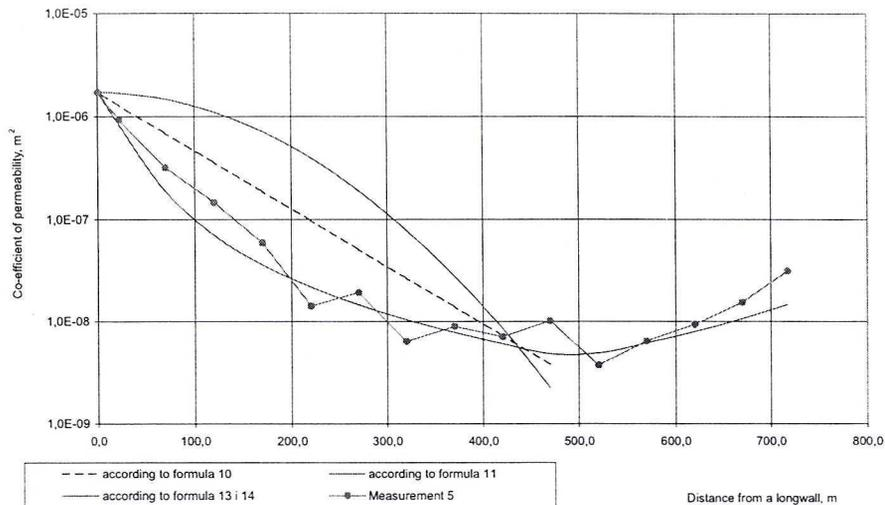
Fig. 10. Change in co-efficient of permeability of caving zone for the last series together with approximation for longwall 170
