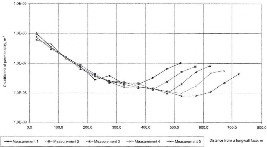
Fig. 6. Change in co-efficient of permeability of caving zone depending on the distance from a longwall face 220
