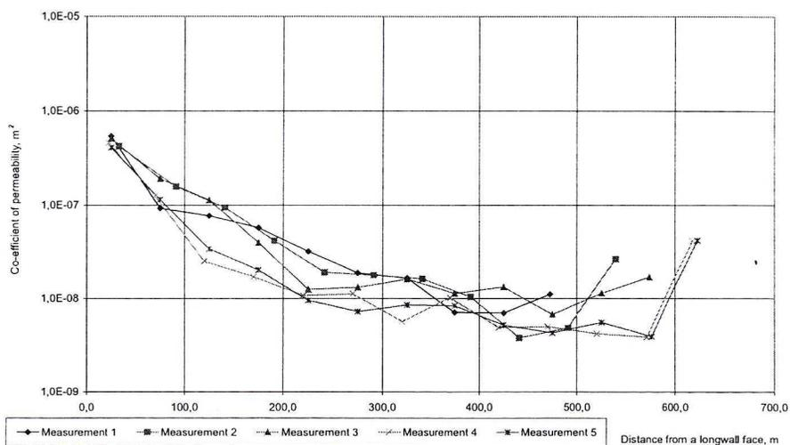
Fig. 3. Change in co-efficient of permeability of caving zone depending on the distance from a longwall face 405
