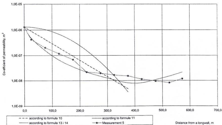
Fig. 11. Change in co-efficient of permeability of caving zone for the last series together with approximation for longwall 660
