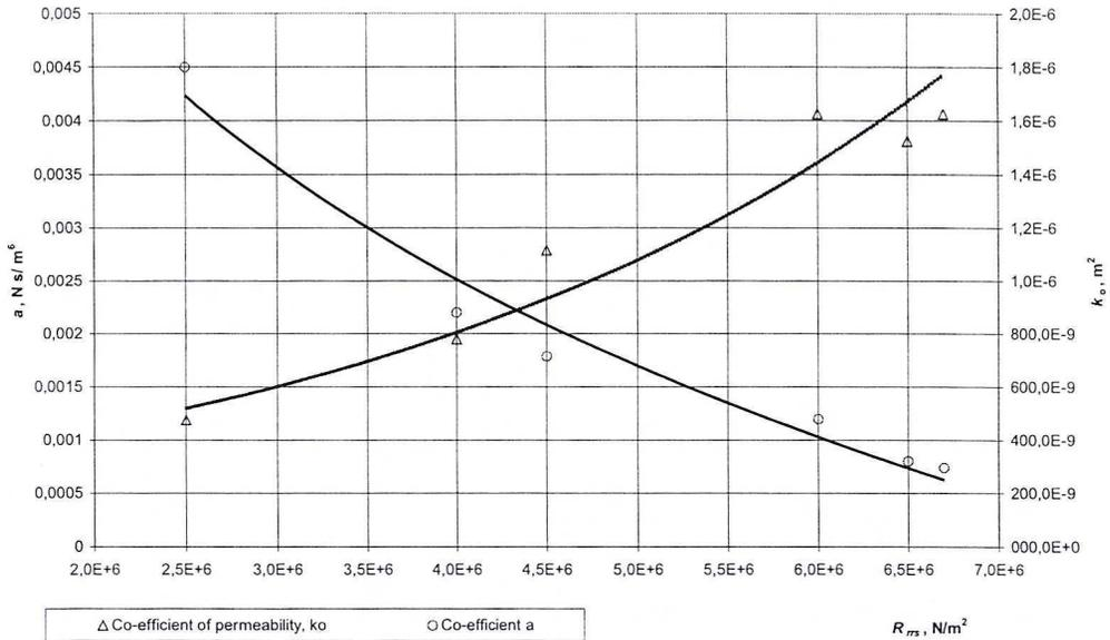
Fig. 14. Dependence of changing of co-efficient of permeability  $k_0$  and co-efficient  $a$  on bed separation resistance of roof rock mass
