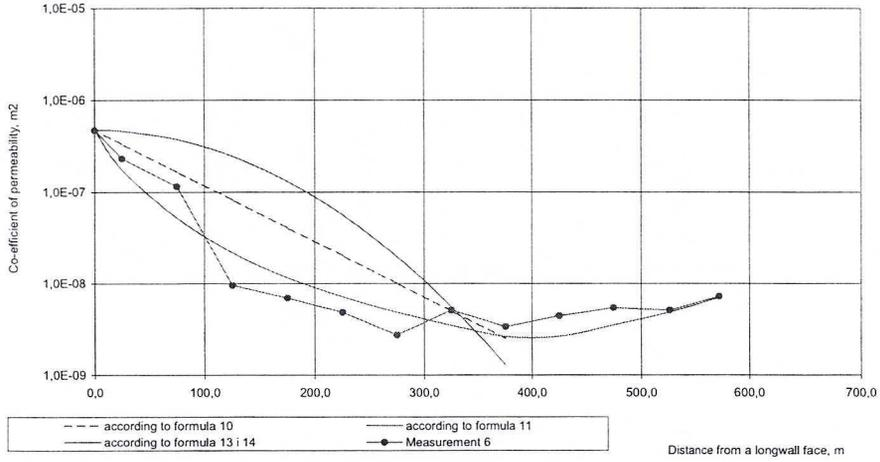
Fig 8. Change in co-efficient of permeability of caving zone for the last series together with approximation for longwall 465
