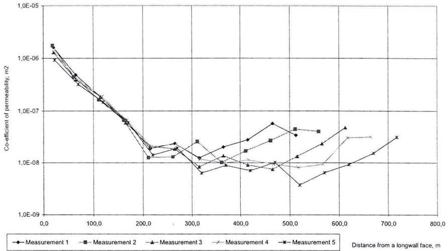
Fig. 4. Change in co-efficient of permeability of caving zone depending on the distance from a longwall face 170
