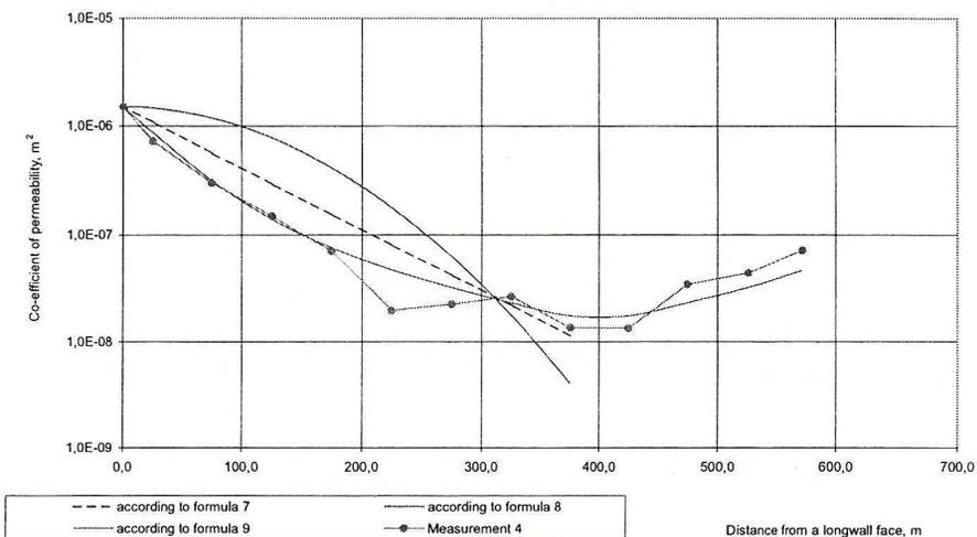
Fig 13. Change in co-efficient of permeability of caving zone for the last series together with approximation for longwall 765
