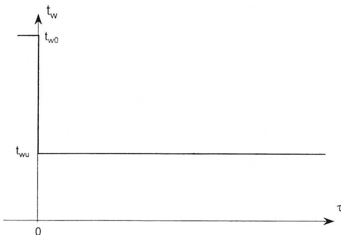
Fig. 4. Time pattern of the temperature of cooling water at the entry to a cooler during its jump fall from value  $t_{w0}$  to  $t_{wu}$
