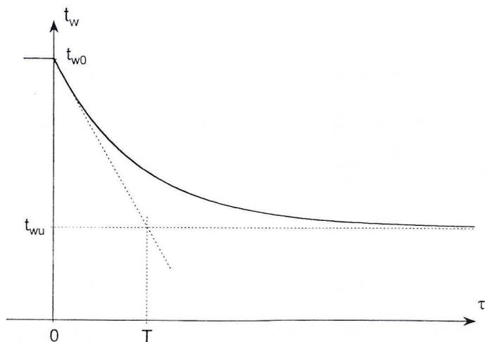
Fig. 2. Time pattern of the temperature of cooling water at the entry to a cooler during its exponential fall from value  $t_{w0}$  to  $t_{wu}$
