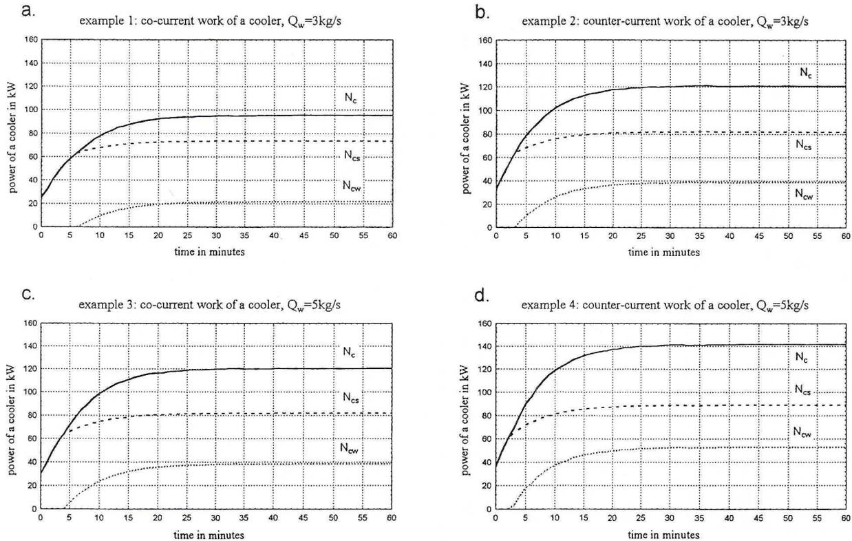
Fig. 3. Power of a cooler in the case of an exponential fall in the inflow temperature of cooling water at time constant  $T = 360$  s from value
