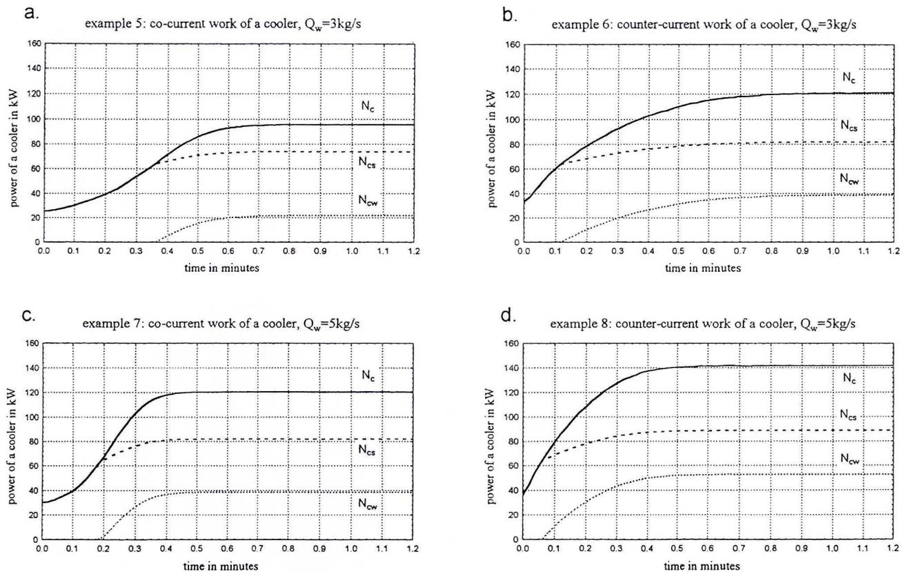
Fig. 5. Power of a cooler in the case of a sudden fall in the inflow temperature of cooling water from value  $t_{w0} = 24^\circ\text{C}$  to  $t_{wu} = 12^\circ\text{C}$
