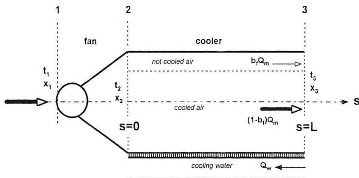
Fig. 1. Scheme of the flow of cooled air and cooling water through
