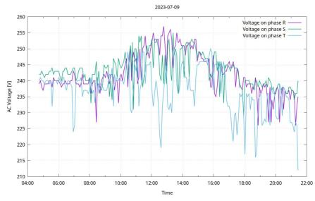
Fig. 6. Voltage waveform on each of tree phase reported by a Sofar SF4ES005 inverter on July 9, 2023.
