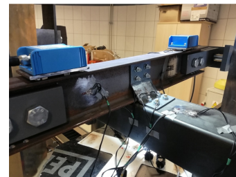
Fig. 8. Inclinometers location on the tested specimen
