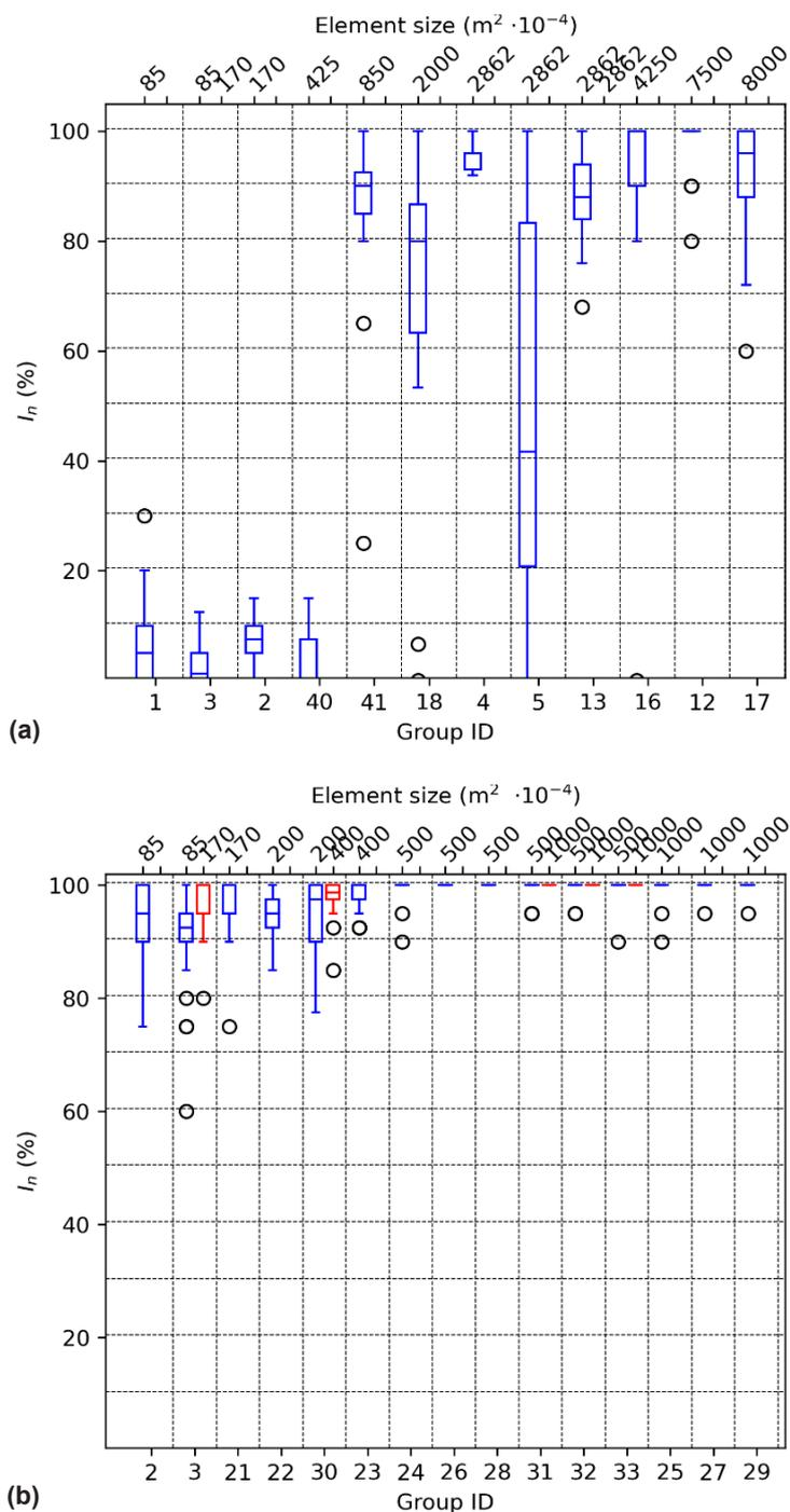
**Figure 3.** Percentage share of collected elements on (a) - sluice gate, (b) - trash racks. Labels on the lower x-axis specify the plastic elements group (as in Table 2 and 3), on the upper one the area of the single plastic element (averaged if two sizes were used); For Groups with two elements, two values of element area were provided (for the sluice gate, only overall statistics for all elements were available, for trash racks statistics for each element size in a group were also provided).
