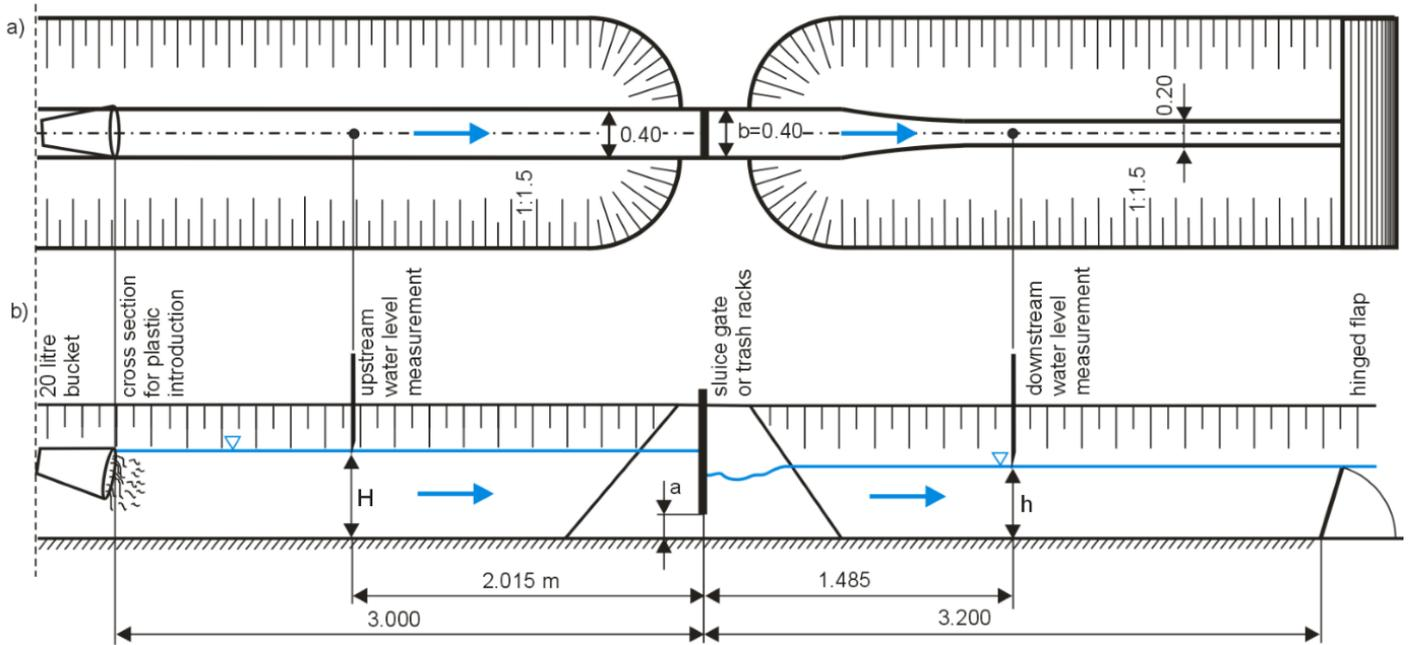
**Figure 1.** The location of measurement points of water levels upstream and downstream sluice gate and trash racks.
